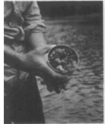
Technology in use for watershed studies in 1957 included this 46-ounce tin can filled with washed gravel. This silt trap was placed in the stream bed on the Harris River as part of the effort to determine whether widespread logging would affect fisheries in southeast Alaska, (luneau 559)
