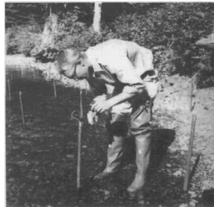
William McNeil demonstrates a method for obtaining dissolved oxygen samples from stand pipes in a creek in 1958. (luneau 851)
