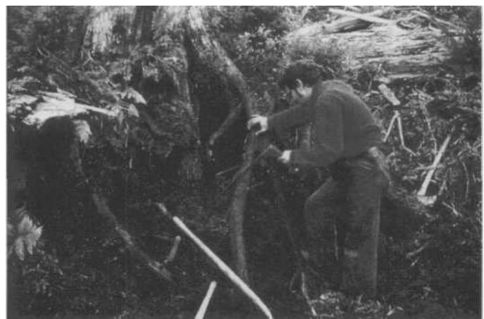
Doug Swanston, shown here testing soil shear strength, was recruited in 1962 to address concerns about soil mass movements on areas of the Maybeso Experimental Forest clearcut in the 1950s. (Schmiege collection)
