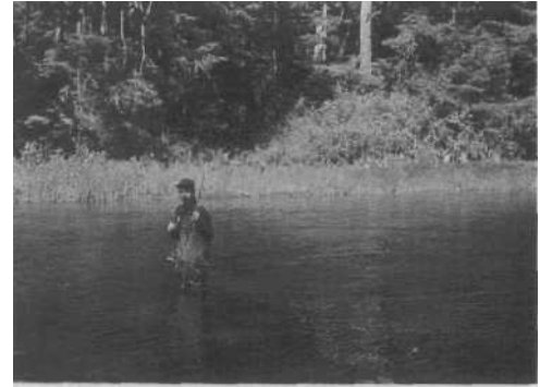
Lawrence Zach taking a discharge measurement with a Price Current Meter #2400, waders, and a tag line. (Juneau, unnumbered)
