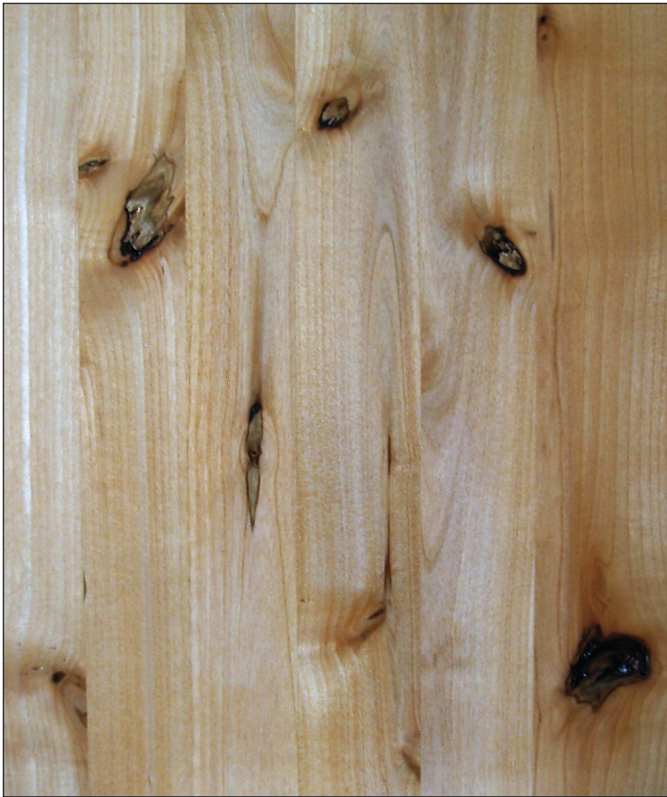
Figure 2—Panel 4: red alder edge-glued panel (high level of character-marked wood).
