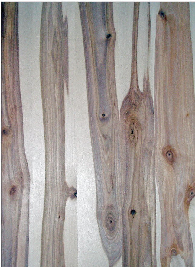
Figure 1—Panel 11: paper birch edge-glued panel (high level of natural stain).
