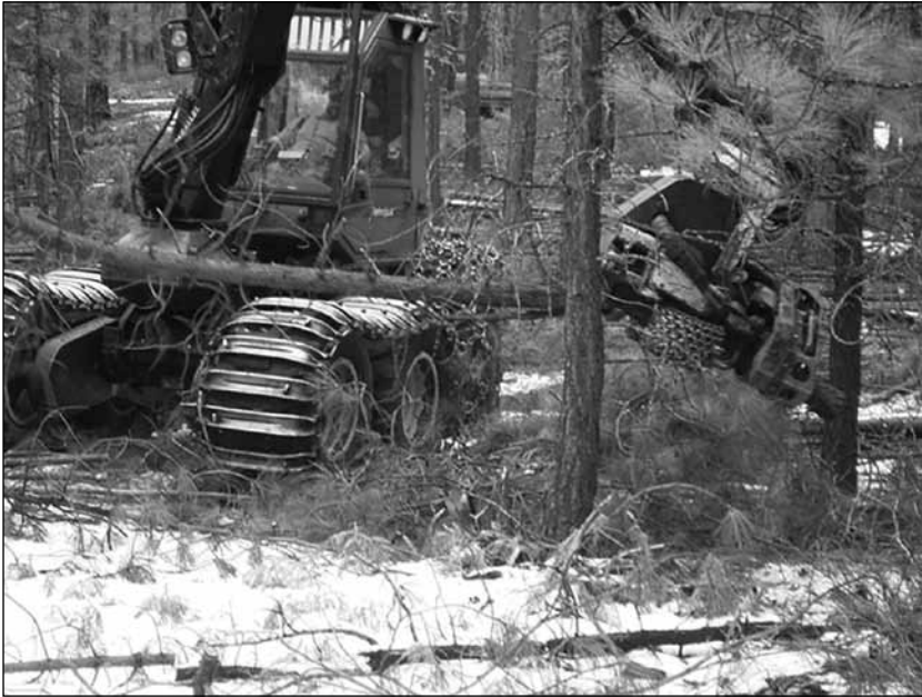
Figure 11—The Timberjack cut-to-length harvester used at Black Butte (app. 7).
