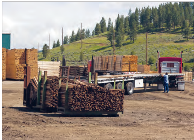
Figure 12—Thanks to American Recovery and Reinvestment Act funding, Evergreen Forest Products was able to invest in dry kilns and a restacker, which enables them to double the amount of wood hauled per truckload to the planing mill.
