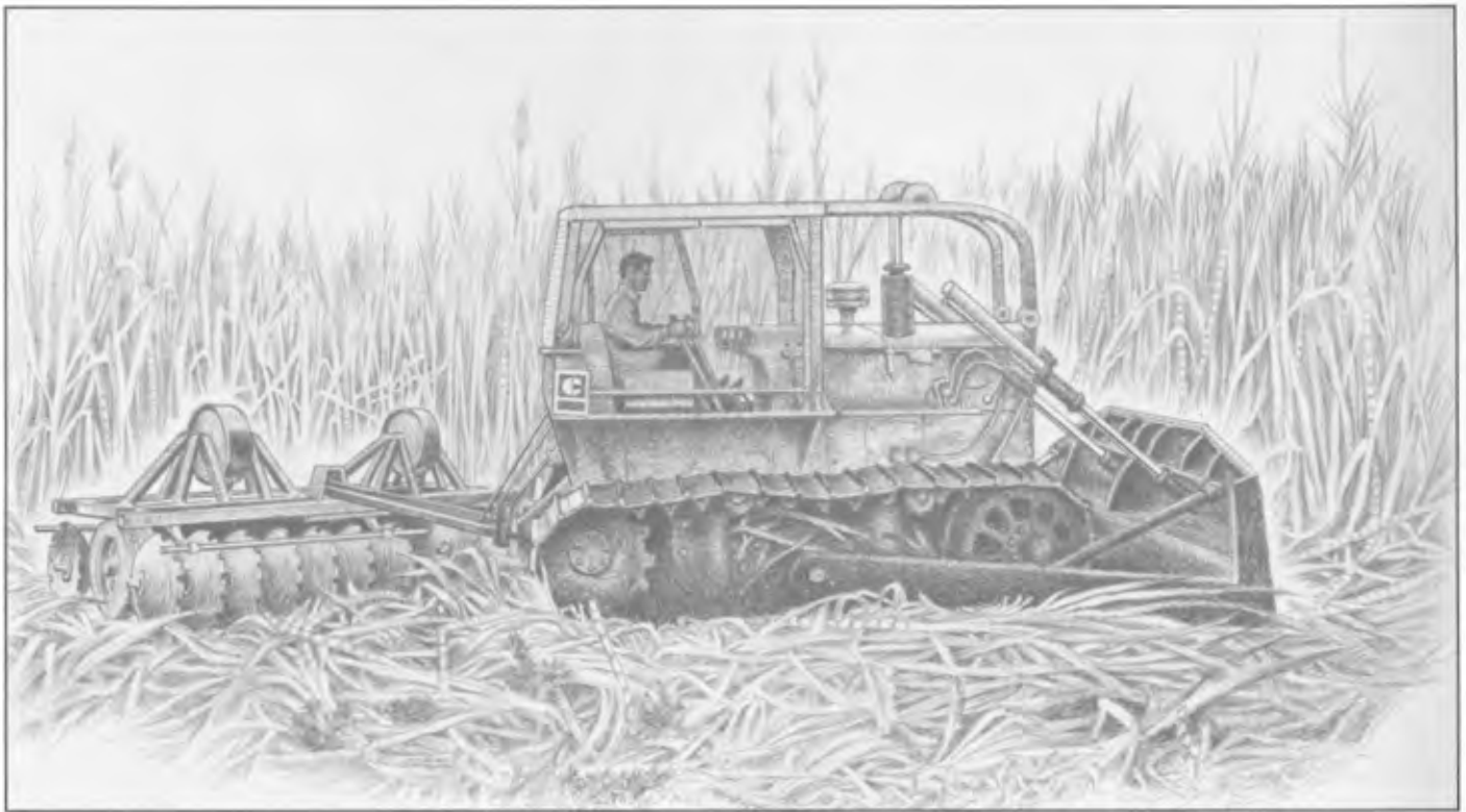
Figure 7 —D-6 tractor pulling cutaway harrow to clear abandoned caneland.
