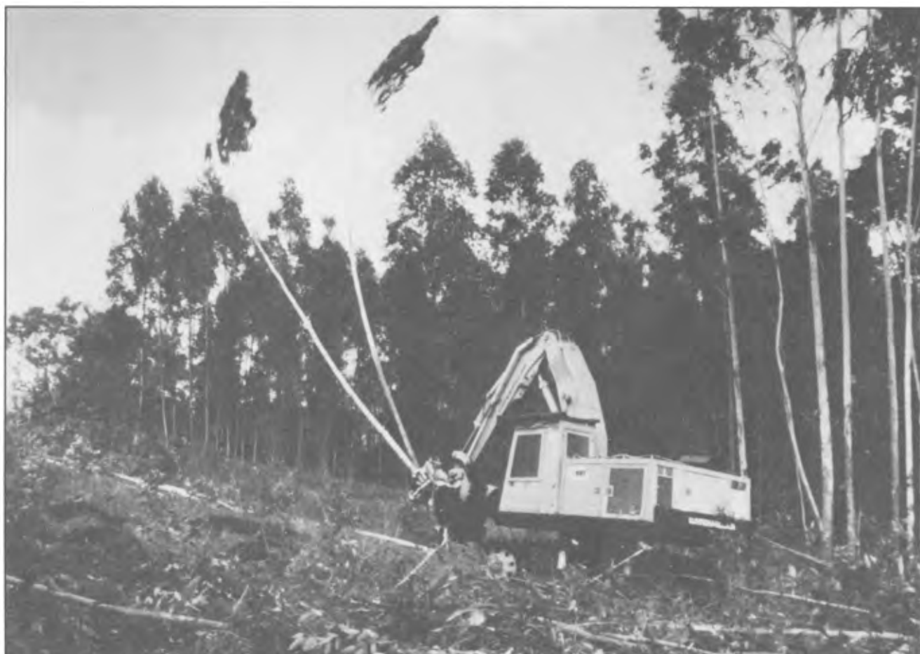
Figure 19 —Harvesting using Caterpillar 227 fitted with feller-buncher head.
