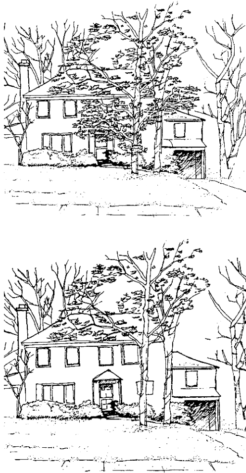
Figure 25. Trees south of a home before and after pruning. Lower branches are pruned up to increase heat gain from winter sun (from Sand 1993).
