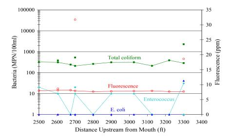
**Figure 5**—Upstream transect on Mill Creek showing longitudinal trends. These samples were taken on 11/17/08 with 0.0 in of rainfall in the previous three days. Note that points without lines indicate seeps or tributaries draining into the main channel.
