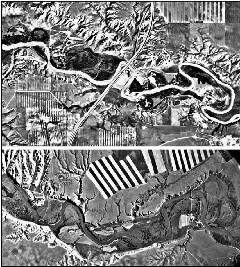
Fig. 2. Two reaches of the Marias River of northern Montana show the reduction in the extent and complexity of habitats related to dams. Upper image: 1991 aerial photograph of a 5.7 km reach of the river upstream from Tiber Dam, showing an unregulated portion of the stream with a substantial active area and complex functional surfaces. Lower image: 1991 aerial photograph of a similar 7.2 km reach of the river downstream from Tiber Dam showing deactivated flood-plain areas and a simple suite of functional surfaces. Tiber Dam, built in 1956, has a storage capacity 1.6 \text{ km}^3 (1,424,000 ac ft); the river has an annual yield of 0.8 \text{ km}^3 (611,700 ac ft). Source: U.S. Geological Survey, EROS Data Center, Sioux Falls, S.D.
