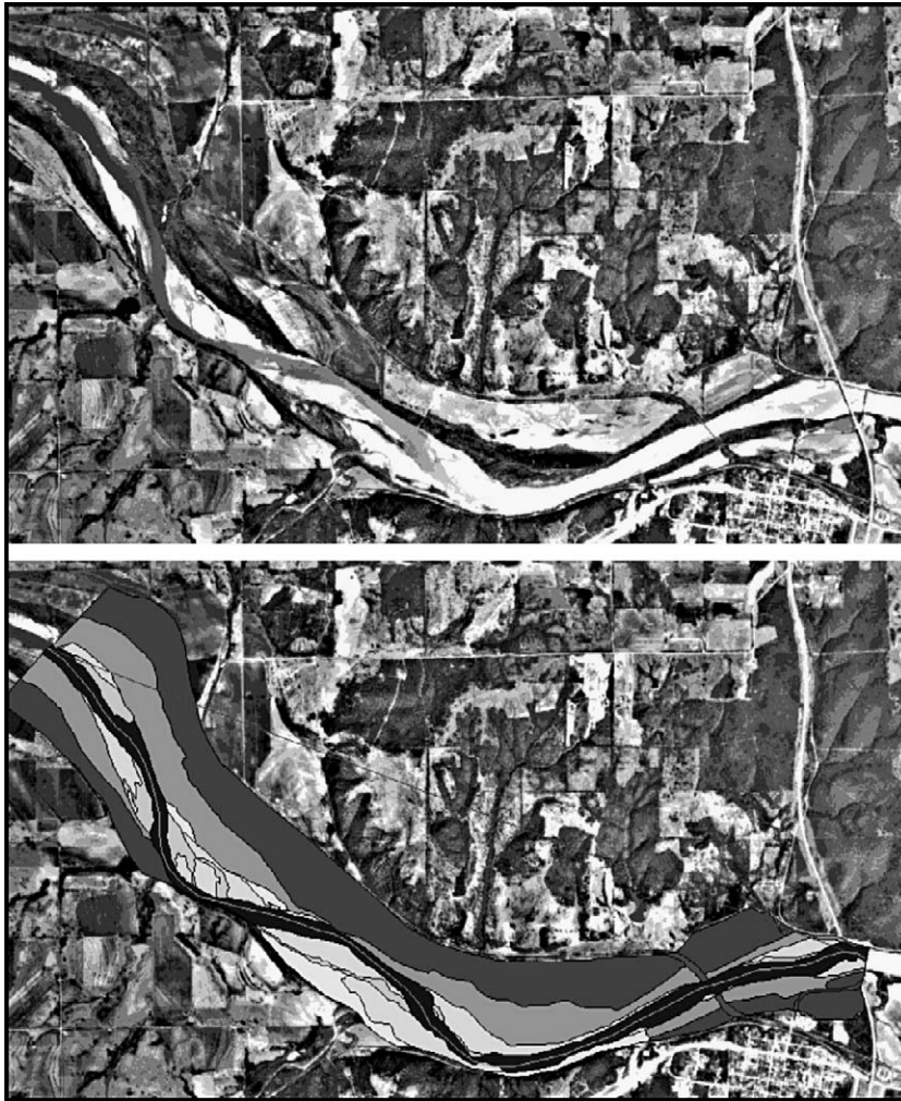
Fig. 8. Mapping of functional surfaces is by on-screen digitizing of an aerial photograph, exemplified by two images of a reach of the Canadian River upstream from Eufala Dam in eastern Oklahoma. The upper image, a 1995 aerial photograph, serves as the basis for a functional surface map showing in the lower image. Sources: aerial photograph from U.S. Geological Survey, mapping by author.
