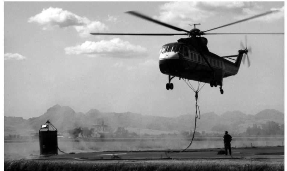
Figure 1—Siller Brothers S-61N helicopter using the 1000-gallon Griffith helibucket.
