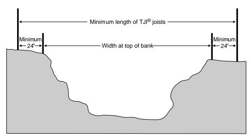
Figure 3—Field measurements needed to determine length of platform required.
