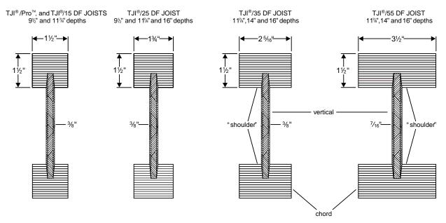
**Figure 2**—Some types of TJI<sup>®</sup> joists that are available; the drawing is based on specification sheets from Trus Joist MacMillan. Chord refers to the pressed wood support along the top and bottom of the joist. Shoulder refers to the interior portion of the chord where pressed particle board (the vertical) connects to the chord.
