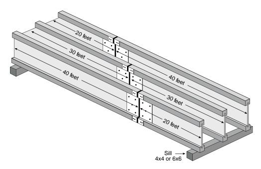
**Figure 7**—An example of lengths of joists and splices used in constructing a platform 60 feet in length. Note that the positions of the splices are offset across the frame of the platform.
