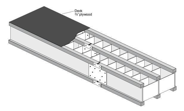
**Figure 9**—Joists, spacers (either 2 x 4s or plywood rectangles), and plywood deck (cut away) used in constructing platform.
