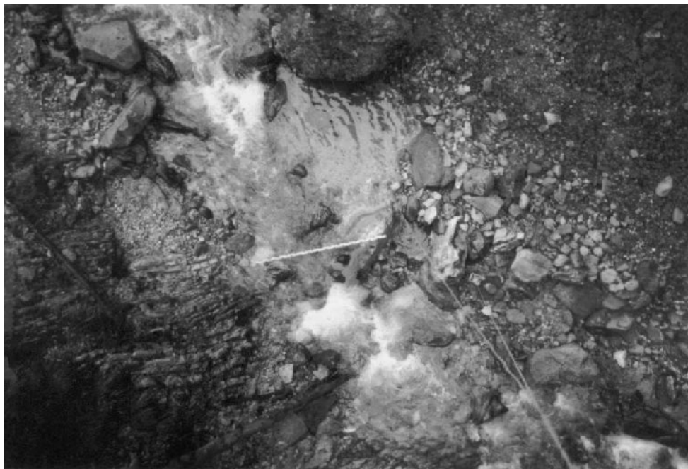
Fig. 4.14: Areal view of a step-pool reach at the Schmedlaine, Bavaria (FRG) taken with a 35-mm camera mounted to a tethered helium balloon. Balloon height is about 15 m. Length of surveyor's rod is 3 m. Flow direction is from upper left to lower right. (Photograph courtesy of B. Kozłowski and P. Ergenzinger, Dept. of Physical Geography, Free University of Berlin, Germany).
