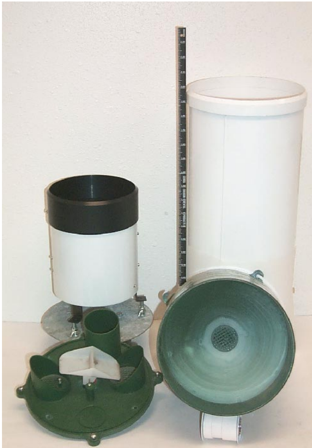
Figure 3 —Three commercially available tipping bucket rain gauges (see appendix B for suppliers).
