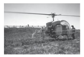
Figure 40—Helicopter equipped with a boom sprayer.
