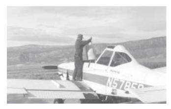
Figure 23—Loading seed into a fixedwing aircraft seed hopper.
