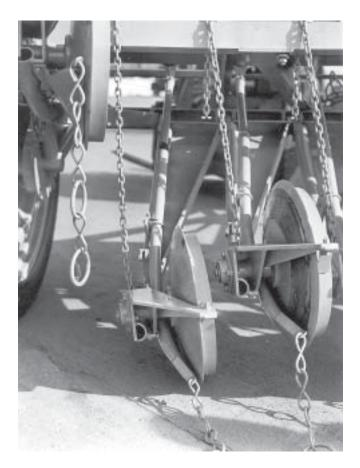
**Figure 14**—Individually suspended arm on a Rangeland drill. Disk furrow openers are equipped with depth bands and a drag chain.
