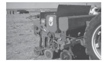
**Figure 17**—Tye drill with four seed boxes and drops. Individual species or groups of species can be seeded at differing depths and rates and with or without press wheels.
