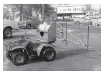
Figure 38—Boom sprayer mounted on an all-terrain vehicle.
