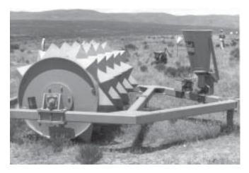
**Figure 12**—Land imprinter equipped with an electric broadcast seeder.
