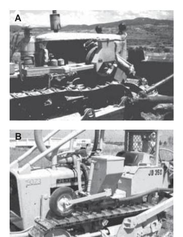
**Figure 27**—(A) Seed dribbler and (B) thimble seeder mounted on the fender of crawler tractors. The Drive wheel meters seed onto the tractor track which moves the seeds forward and deposits them on the ground. Tractor weight buries the seed in a firm seedbed.
