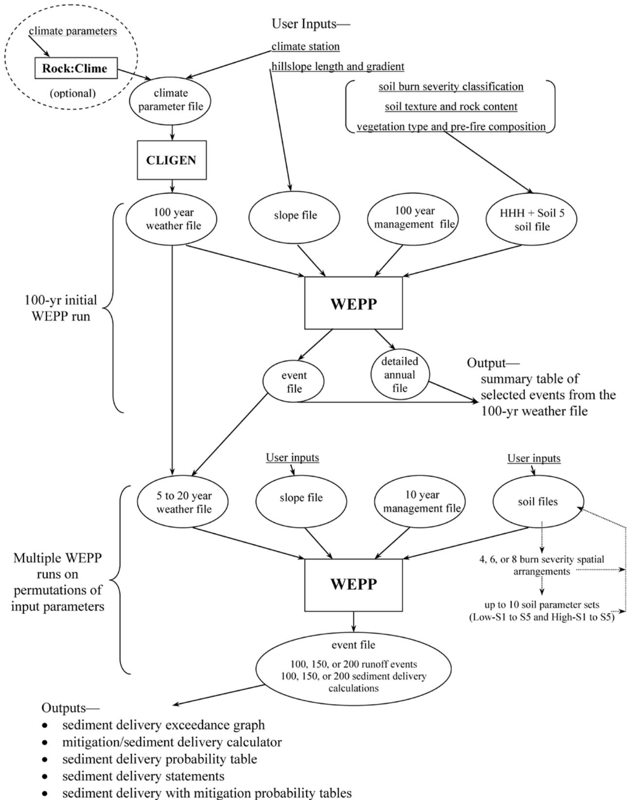
**Figure 5.** Flow chart of the ERMiT modeling process used to calculate probabilistic sediment delivery using the CLIGEN weather generator and the WEPP erosion prediction engine.
