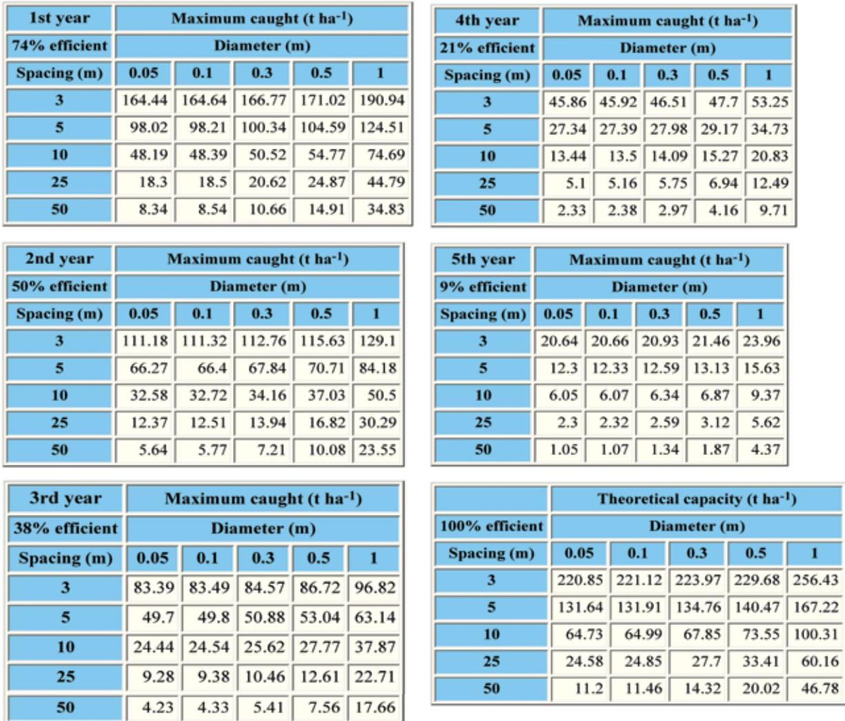
Figure 17. ERMiT erosion barrier efficiency calculator.
