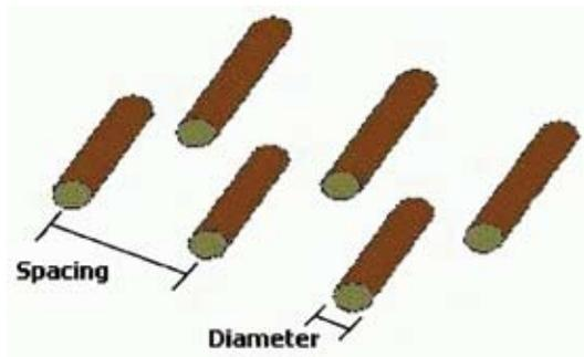
**Figure 7.** Erosion barrier diameter and spacing between rows.
