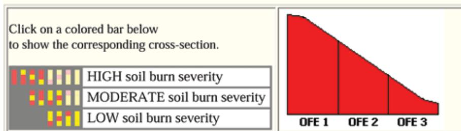
**Figure 6.** Graphic viewed by clicking on “explain” from the soil burn severity class box. The bold colored squares (red is high and yellow is low soil burn severity) represent the upper, middle, and lower OFEs that are modeled for the first year following a fire. The faint colors indicate OFE arrangements modeled in subsequent post-fire recovery years.
