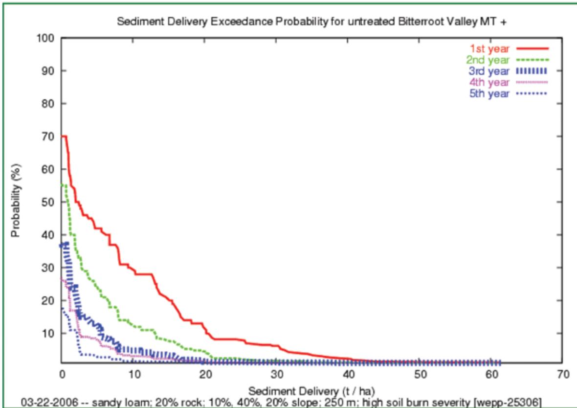
**Figure 11.** Output graph showing exceedance probability versus event sediment delivery for five years after the fire from the modeled, untreated hillslope.
