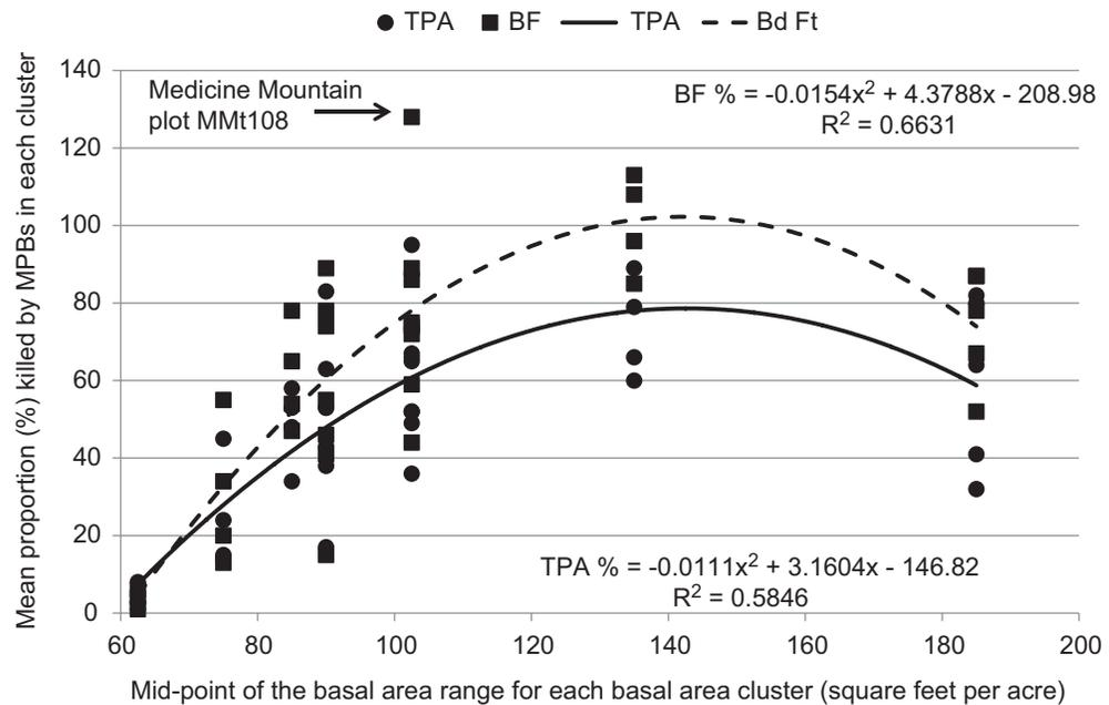
**Figure 141**—Relationship between tree density estimated by square feet of basal area per acre and the mean proportion of both trees and board feet per acre killed by MPBs within each basal area cluster.
