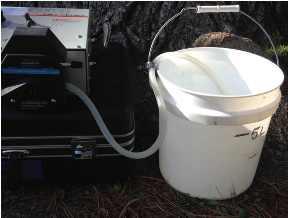
Figure 1 —Outflow end of tubing threaded through hose clamp and placed into outflow bucket.
