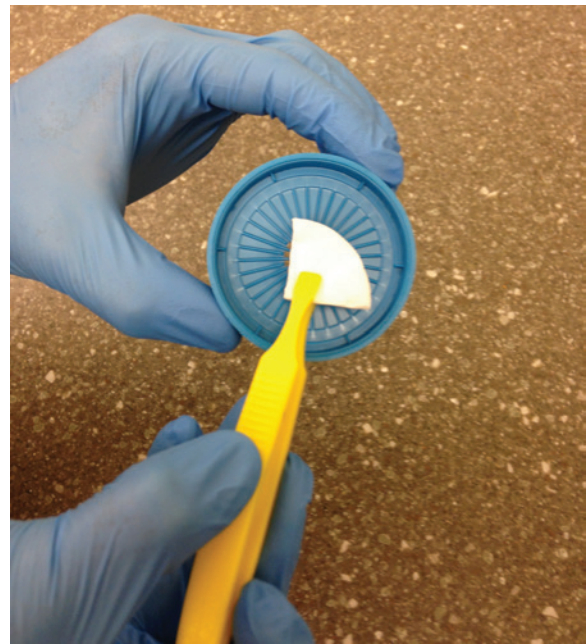
Figure 5 —Folding the filter paper, filtrate (usually brown) side in.
