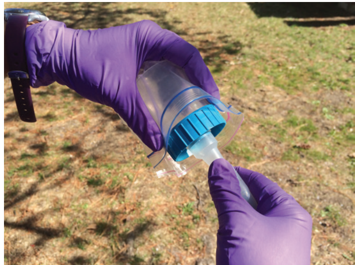
Figure 2 —Attaching the filter assembly to the adapter while using the packaging bag.
