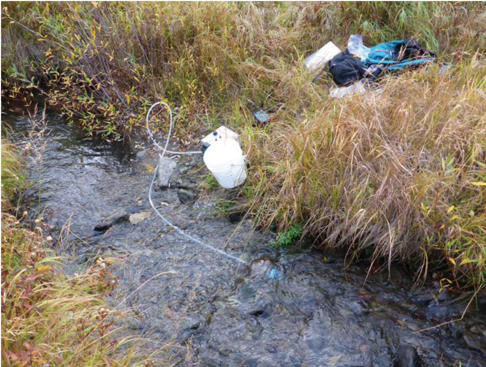
Figure 3 —Collecting a field sample. Filter cup is submerged in the main current upstream from the pump and bucket. In this case, the cup is held in place in the current with a rock.
