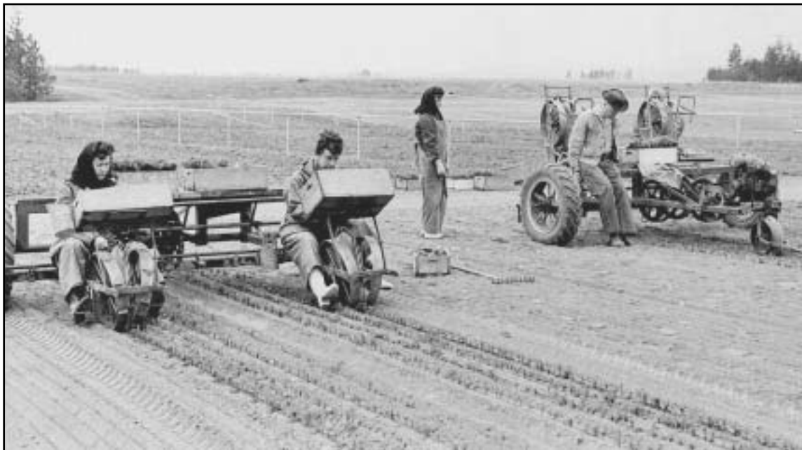
Figure 7. One of the first machine transplanters that was modified for tree nurseries was self-propelled and transplanted two rows at once.
