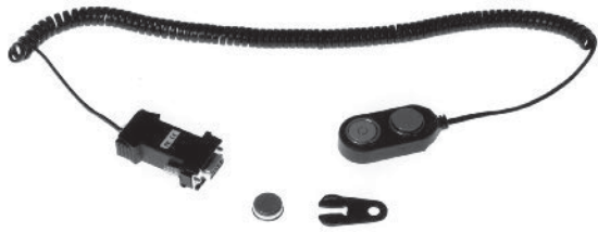
Figure 1. The ThermoChron iButton, the size of 2 stacked dimes, measures time and temperatures of seedling bundles while they in storage or being transported.
