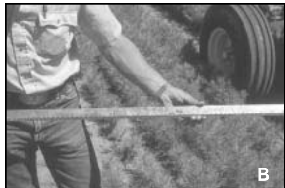
Figure 5 A/B. The New Zealand root pruner (A) featured a thin oscillating blade (B) which precisely prunes roots and produces a seedling with transplant characteristics.
