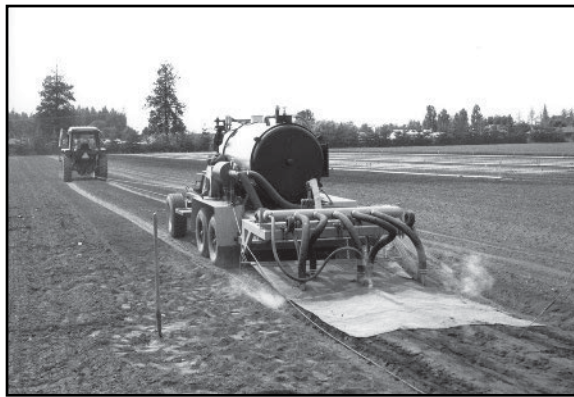
Figure 4. MTDC developed this prototype machine to inject steam into nursery beds, sterilizing the soil as an alternative to using pesticides. It proved to be too slow for production use.
