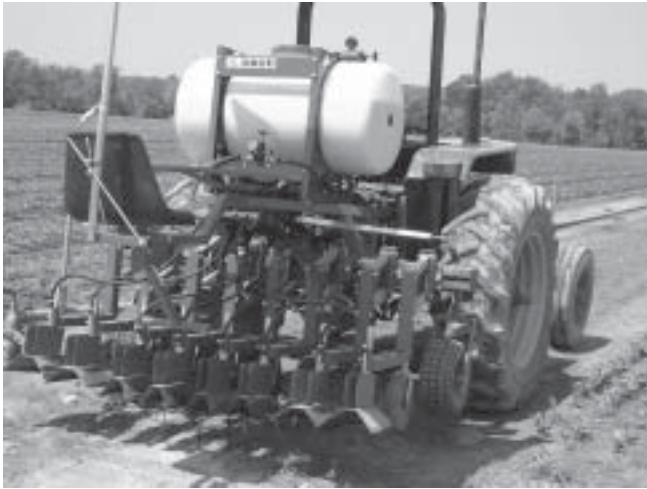
Figure 1 —Egedal shielded sprayer used to spray Roundup™ directly to weeds between drill rows.
