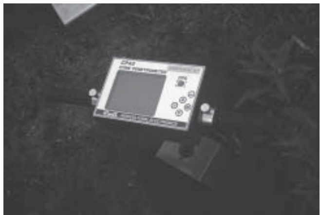
Figure 2 —New-generation soil penetrometers are easy to use, and save readings for further analysis back at the office.
