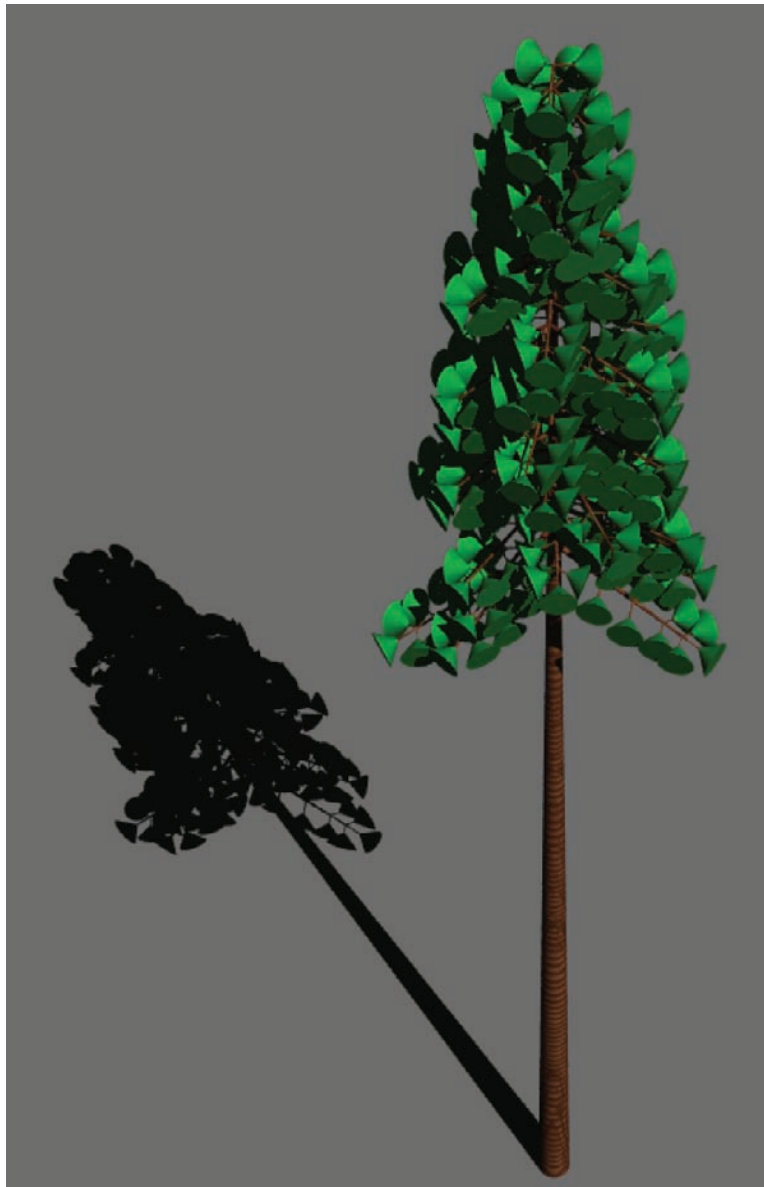
Figure 11 —Visualization of a medium sized ponderosa pine tree modeled with FUEL3-D. The shadow of the tree, modeled with ray-tracing procedures, is shown at left.
