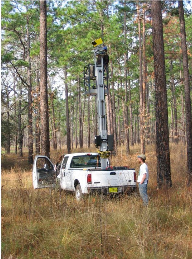
**Figure 1**—A ground-based LIDAR system: The MTLS (Mobile Terrestrial Laser Scanner) is used to mobilize Optech's ILRIS 3<sub>6</sub>D (yellow instrument) for collecting high-resolution 3D point-cloud laser data.
