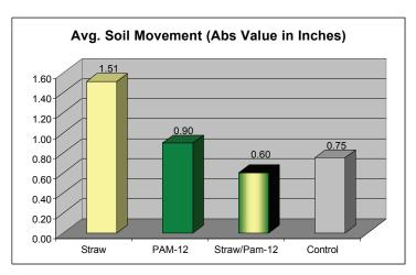
Figure 2—Erosion control test results on four treatments.
