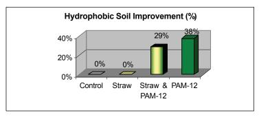
**Figure 1**—Comparison of four treatments and the hydrophobic soil improvement.
