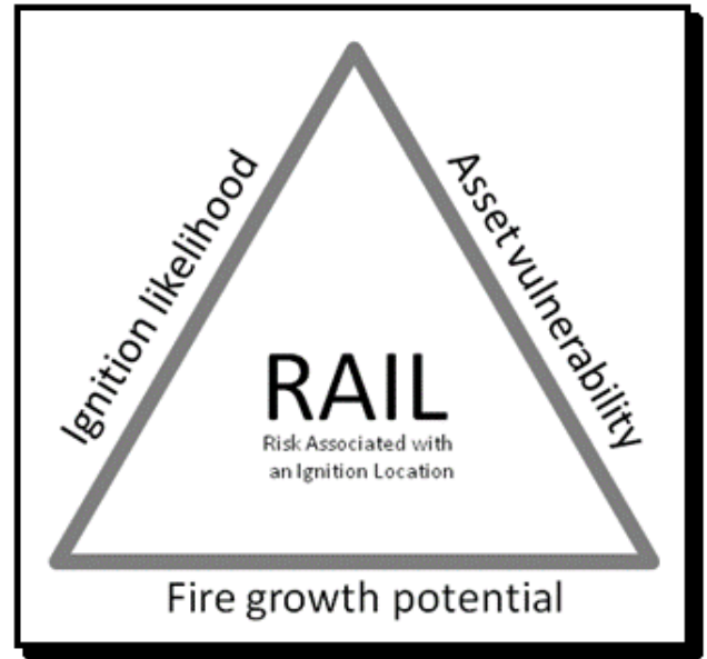
Figure 10 —RAIL analysis triangle. The wildfire risk associated with an ignition location is a function of the likelihood of ignition at the location and the fire growth potential and the vulnerability of resources and assets in the area surrounding the location.
