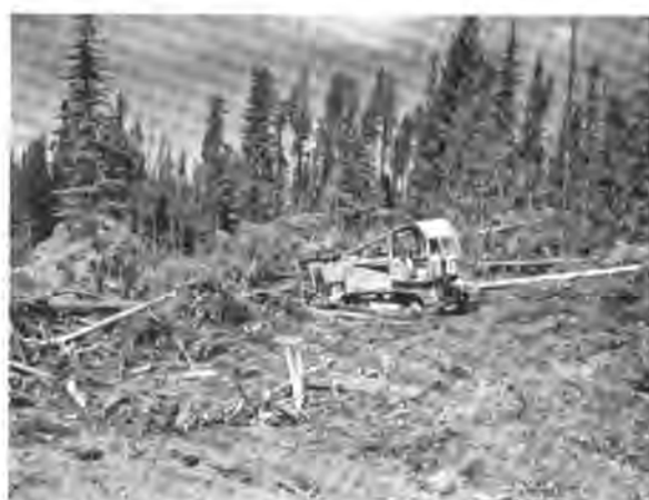
Figure 22.—Mechanical scarification using a brush blade mounted on a bulldozer, Kootenai National Forest. Logging slash and brush are pushed into piles or windrows and burned.
