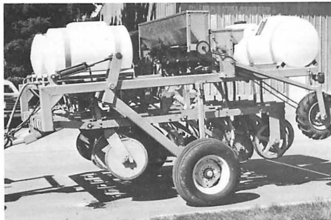
Figure 4—Rangeland slot seeder.
