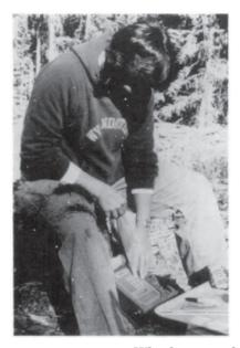
pling soils from the bottom upwards, after they have been "cleaned" from the top downwards. Usually a 100 g sample is sufficient for most analyses, but more should be taken if the soil is particularly stony. Make sure that your sample represents the pedon.
