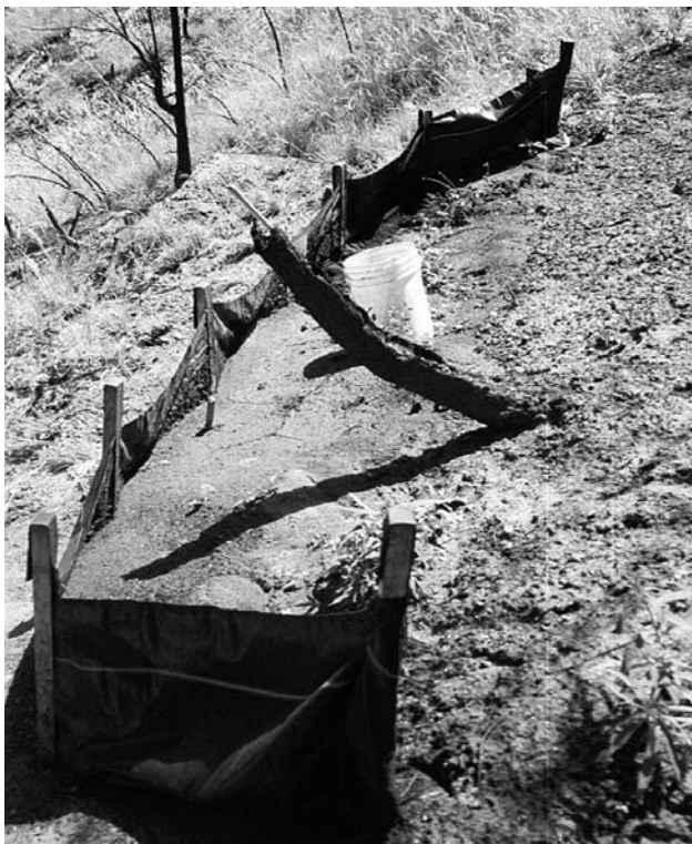
Figure 3. Photograph of 800 kg of eroded sediment trapped in the silt fence at Site 2-plot A after the 15 Jul 01 rain event
