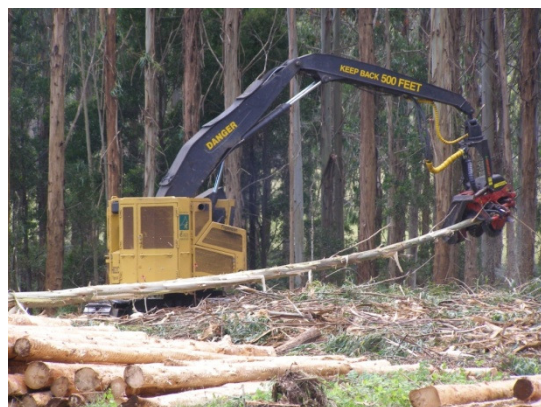
Figure 4.2: Tigercat tracked harvester delimbing and topping a felled Eucalyptus nitens stem during a streamside harvesting study on the effectiveness of Best Management Practices. Note the slash coverage remaining in the harvested area. Photo credit: Daniel G. Neary
