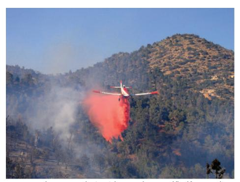
Figure 2. A single-engine airtanker (SEAT) drops retardant on a wildland fire near Caliente, Nevada. Photo by Tim E. Wallace, USDA Forest Service.
