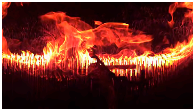
Movie S4. Close-up view from high-speed movie shows forward flame bursts and peak and trough flame structure at the leading edge of an approaching fire in the MFSL wind tunnel burning engineered cardboard fuel bed.
