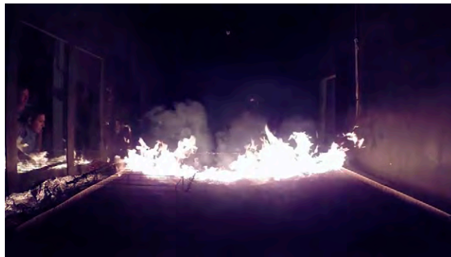
Movie S3. Low-speed movie of experimental burn in cardboard fuels uses smoke to visualize vorticity of the airflow behind the approaching flame zone.
