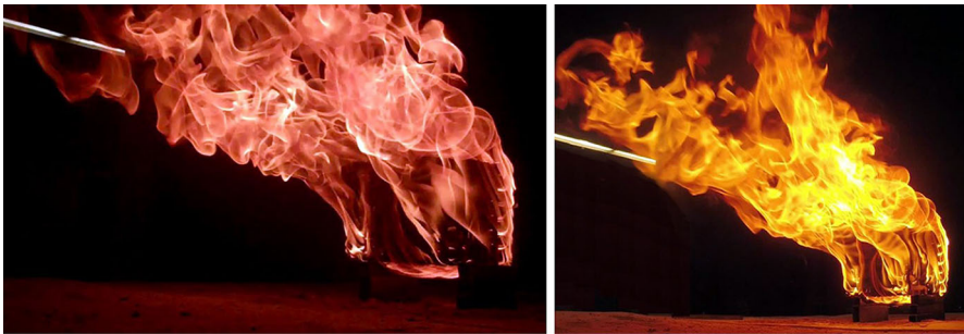
Figure 5. Flame structure from crib design #3 with 0.37 m/s (left) and 0.7 m/s (right) wind speed.
