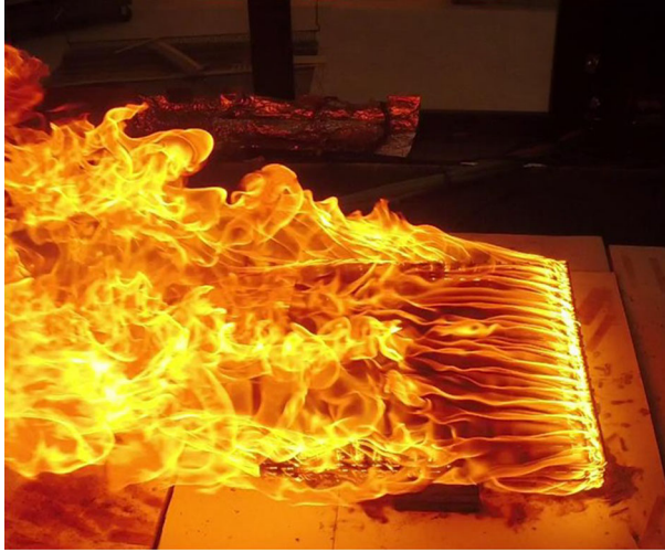
Figure 9. Flame structure from crib design #7 with 0.7 m/s wind speed.
