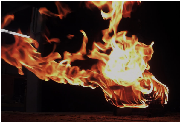
Figure 8. Flame structure from crib design #6 with wind speed of 0.7 m/s.
