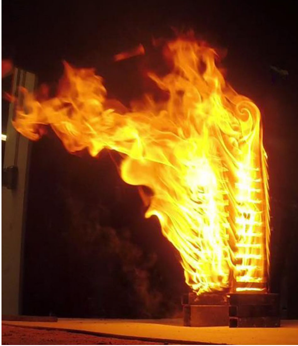
Figure 4. Flame structure from crib design #1 with 0.7 m/s wind speed.
