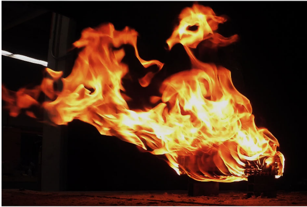
Figure 7. Flame structure from crib design #5 with wind speed of 0.7 m/s.
