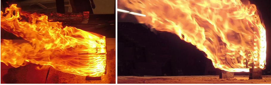
Figure 6. Flame structure from crib design #4 with 0.7 m/s wind speed.
