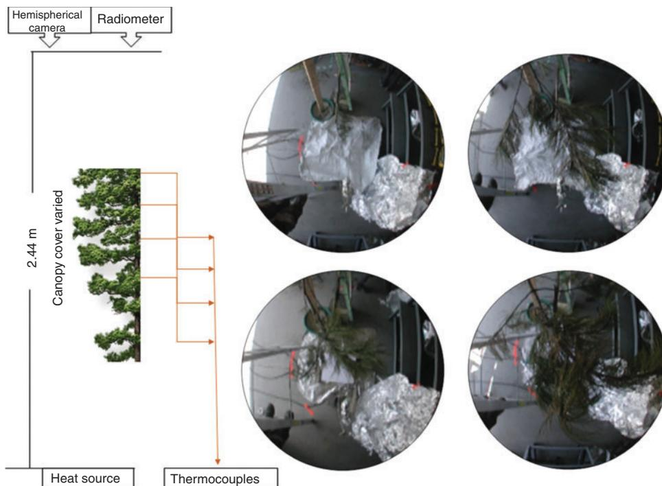
**Fig. 1.** Schematic drawing of the experimental setup in the laboratory and hemispherical photos of different canopy cover levels explored in the laboratory burn experiments. The hemispherical camera was centred over the heat source at the time the photo was taken and the simulated canopy was centred over the heat source during the experiment.
