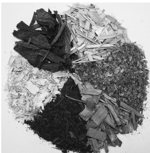
Figure 2.6. Six different woody biomass feedstocks produced at a single sawmill (starting at 12 o'clock and running clockwise from left): dry planer shavings, ground wood fuel (also known as "hog fuel"), screened chips, sawdust, pulp chips and screened bark mulch. Photograph by Nate Anderson.
