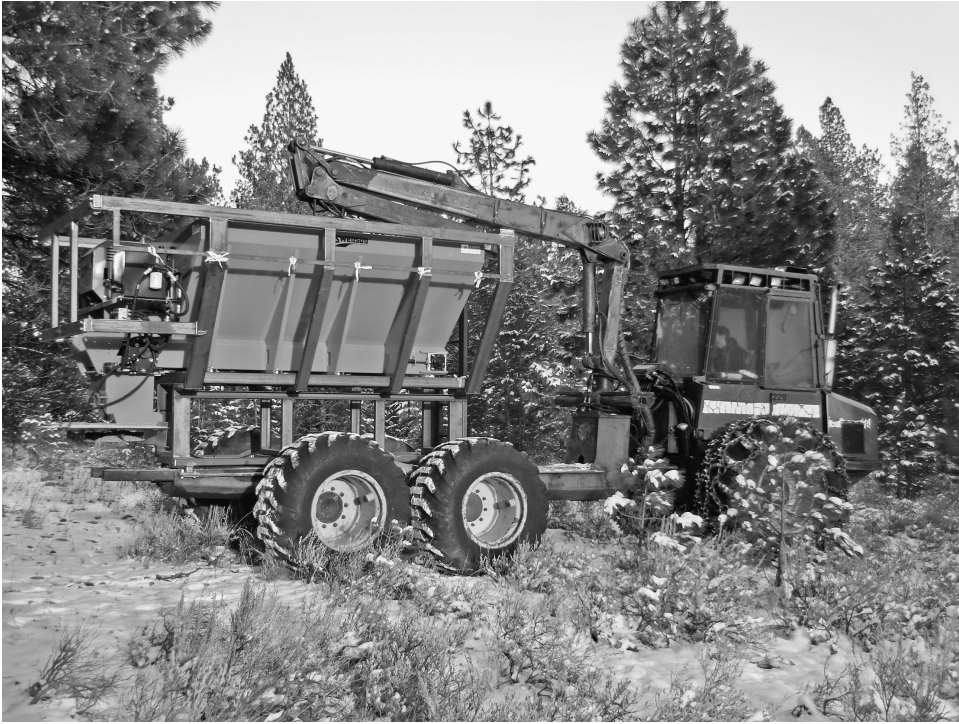
Figure 2.8. A six-wheeled forwarder, normally configured to carry logs, here mounted with a modified pellet spreader to apply biochar pellets on forested sites developed by the Missoula Technology Development Center, Missoula, MT. Photo by Han-Sup Han. (A black and white version of this figure will appear in some formats. For the colour version, please refer to the plate section.)
