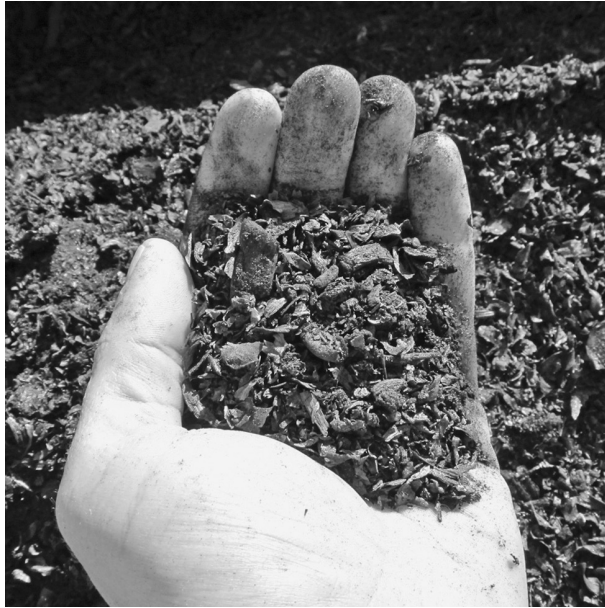
Figure 2.1. Charcoal produced from loblolly pine ( Pinus taeda ) sawmill planer shavings using a high temperature (800–1100°C) pyrolysis system. Based on its feedstock and conversion process, this product will be classified as biochar if it is used as a soil amendment. Photograph by Nate Anderson.
