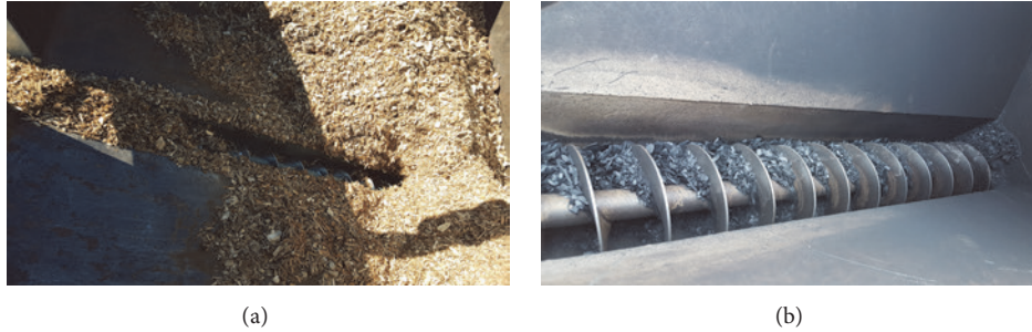
FIGURE 4: Rotating auger moving (a) chips and (b) biochar in the rotary kiln. (Photo credit: S. Bell, retired USDA Forest Service.)
