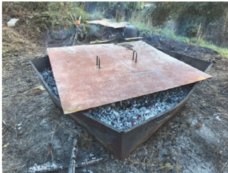
FIGURE 5: Mini kiln with charcoal ready to be covered to create biochar. (Photo credit: D. Morrison, retired USDA Forest Service.)
