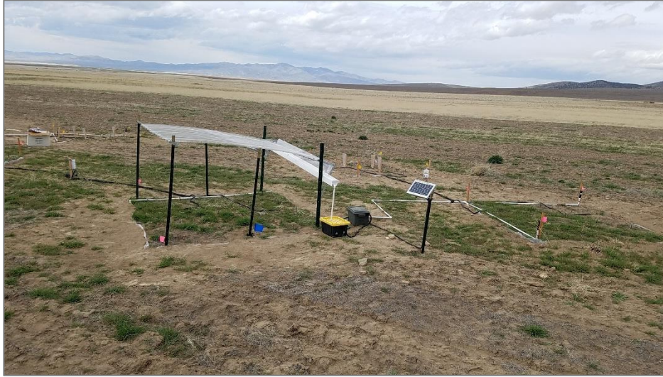
Figure 2 Rainout shelter (left), which collects rain and is added to the rainfall addition plot (right) using an automatic rainfall manipulation system (ARMS). Frame intercepts 50% rainfall and barrel collects rainfall for 50% addition.
