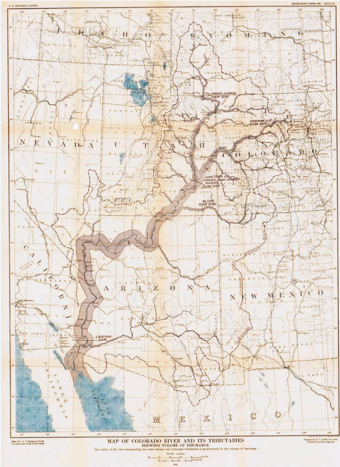
Figure S1-1. Map showing the volume of annual discharge of the Colorado River as estimated by LaRue (1916, plate XX).
