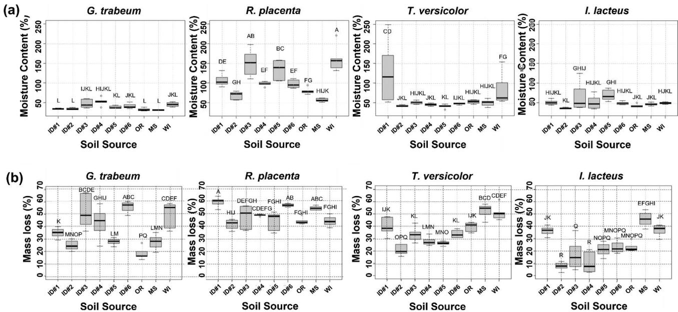
Figure 4.—(a) Moisture contents and (b) mass loss of decayed wood samples after 8 weeks of brown rot (*Gloeophyllum trabeum* and *Rhodonia placenta*) and white rot (*Trametes versicolor* and *Irpex lacteus*) fungal exposure using different soils. The same letter above each bar indicates no significant difference among soil sources at a significance level of 0.05.
