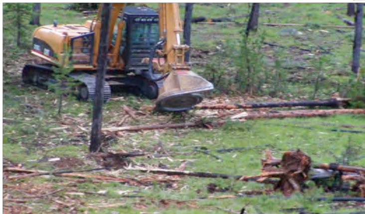
Mechanical treatments reduce understory fuels. These photos show the Warm Lake Highway Project in Idaho before treatment (top), during mulching of surface and ladder fuels (middle), and after treatment (bottom) (photo credit: Graham et al, 2009).
