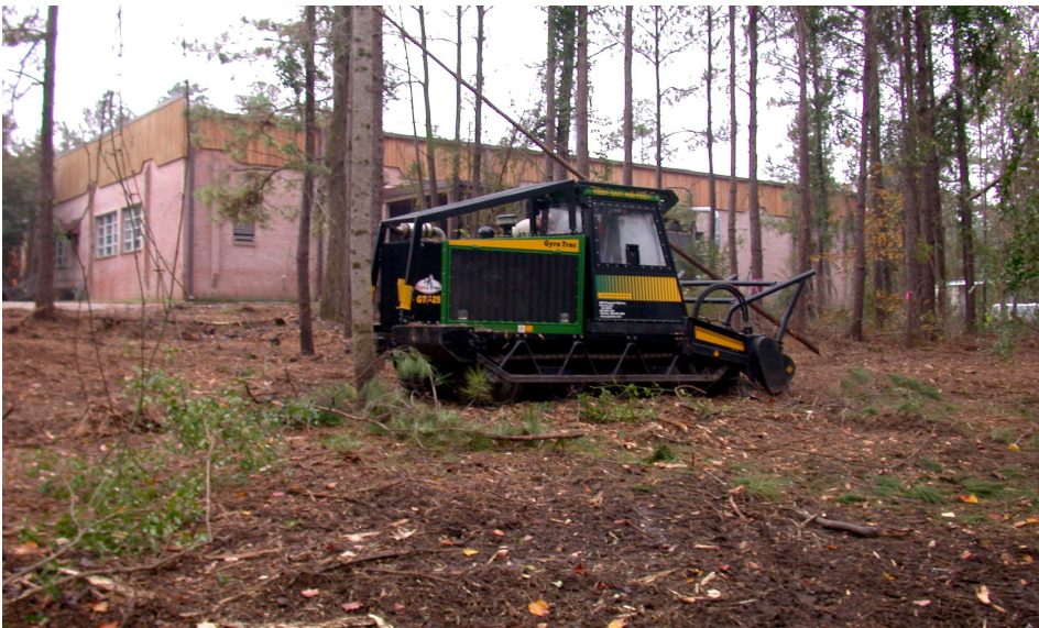
A mastication machine treats surface fuels and provides a fire break surrounding buildings (photo: D. Mitchell, USDA Forest Service, Southern Research Station).
