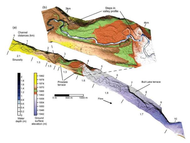
**Figure 4.** (a) Digital elevation model of upper Bear Valley Creek. Digital topography produced from EAARL data gridded to a 3 m interval. Reference distances are measured along the channel and sinuosity is calculated as channel length/straight-line valley distance over the indicated valley segments. (b) Inset showing degraded step in the valley profile at distance about 3,800 m and shorter valley step at about 2,800 m.
