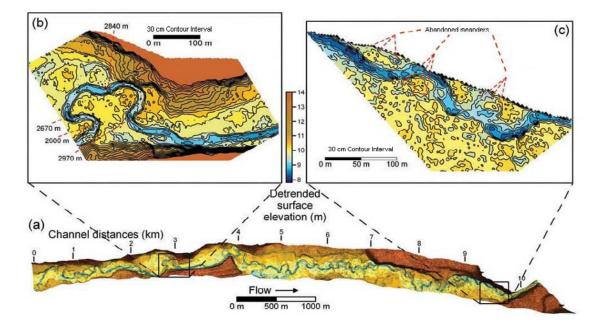
**Figure 5.** (a) Channel, floodplain, and terrace topography after the valley gradient has been removed. (b and c) Contour maps of selected channel reaches, showing the ability of EAARL to simultaneously resolve floodplain, terrace, and channel topography. All digital topography produced from EAARL data gridded to a 3-m interval.
