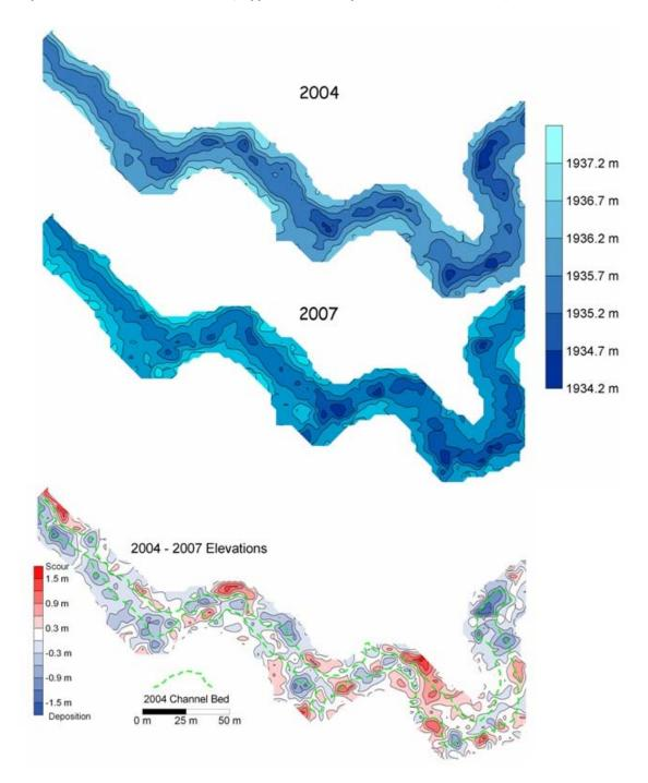
Figure 7. Change in Elk Creek between EAARL surveys in 2004 and 2007. Flow is left to right. The dashed green line shows the limits of the channel bed in 2004 for reference.
