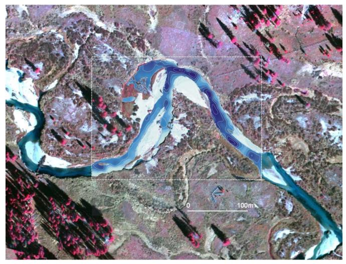
**Figure 8.** EAARL bathymetry of a portion of Elk Creek (bathymetry confined to area of channel within white box) overlaid on a mosaic of digital color-infrared imagery. The color-infrared imagery has not been rigorously ortho-rectified and co-registered to the bathymetry. The imagery and bathymetry were acquired simultaneously by the EAARL system. Bathymetric contours are at 50 cm intervals.
