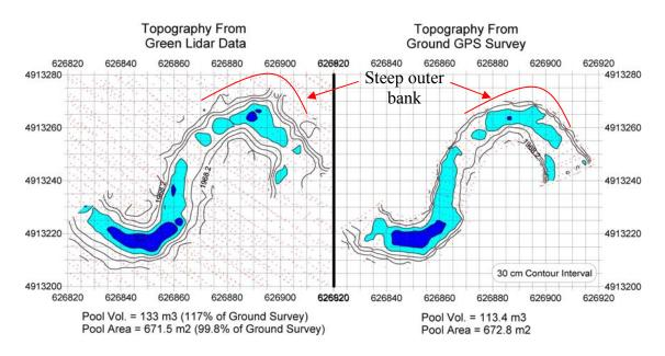
**Figure 3.** Comparison of topography mapped in the same pool-riffle channel reach with EAARL data (left panel) and survey-grade GPS (right panel). Red dots are points were elevation data were collected by each method. Notice the continuous EAARL data acquisition inside the channel and in the surrounding floodplain.
