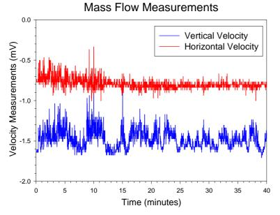
Figure 6 Typical horizontal and vetical measurements from FBP sensors.
