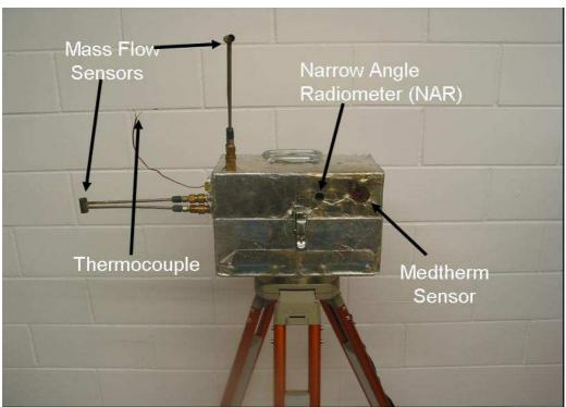
Figure 1 Photograph of Fire Behavior Package.
