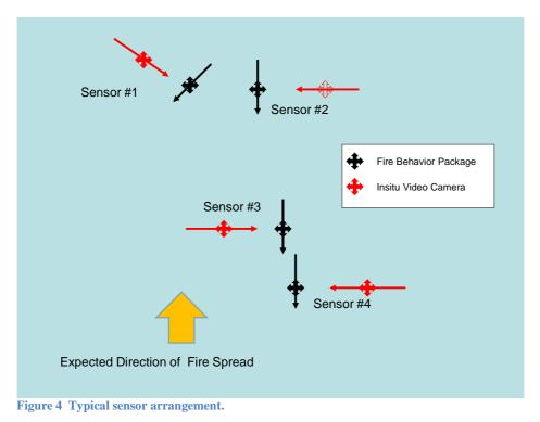
After the enclosures are mounted, positioned and "turned on" a GPS position is recorded for each, including reference orientation (compass direction), height above the ground, and any other local vegetation, or environment information deemed relevant. The insulation is then installed.
