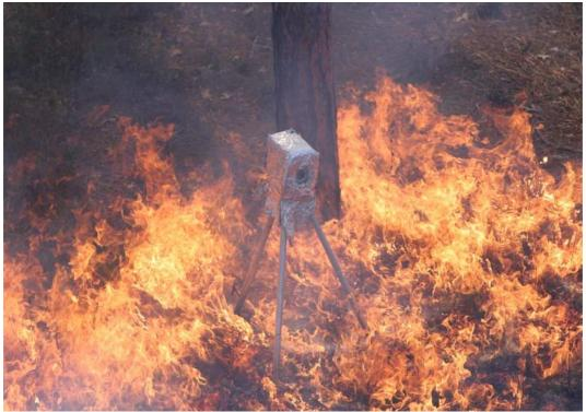
Figure 3 Insitu Video Camera mounted on tripod.
