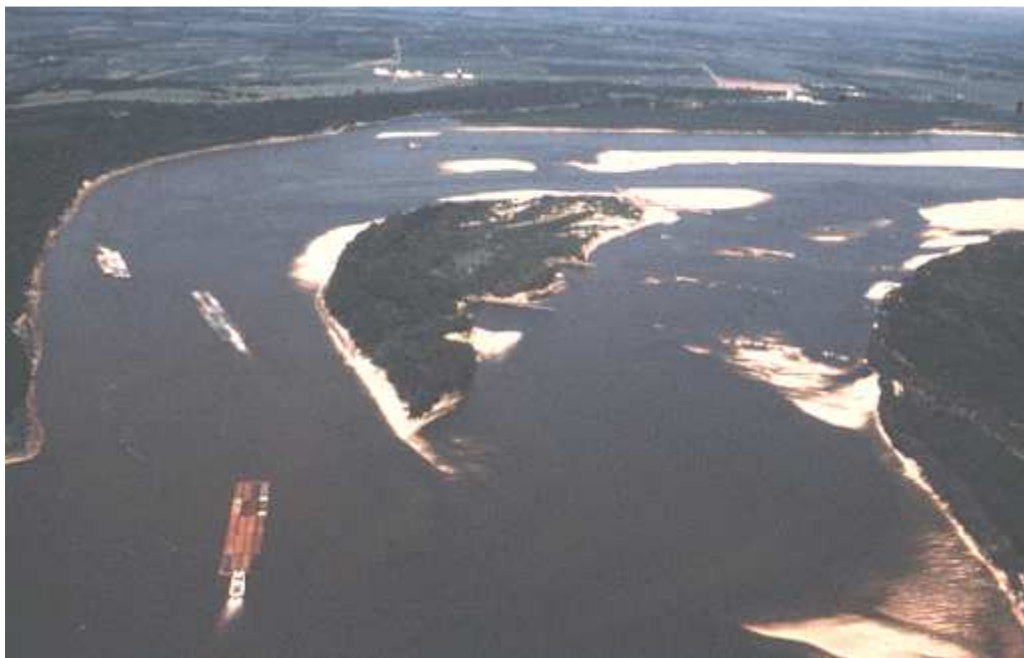
Figure 2.6 Typical Middle Bar (from Watson et al. (2005))
