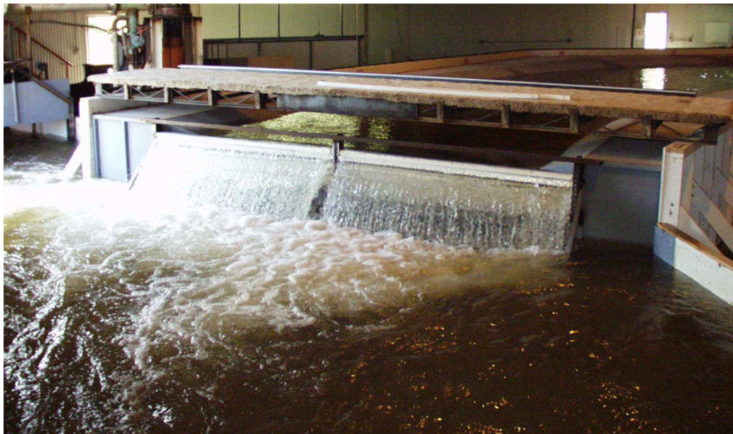
Figure A.20 Stop Log for Calibration of the Model
