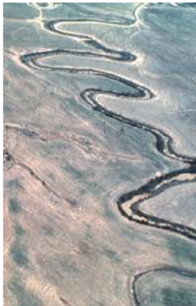
Figure 2.1 Typical Meandering Channel (from Watson et al. (2005))
