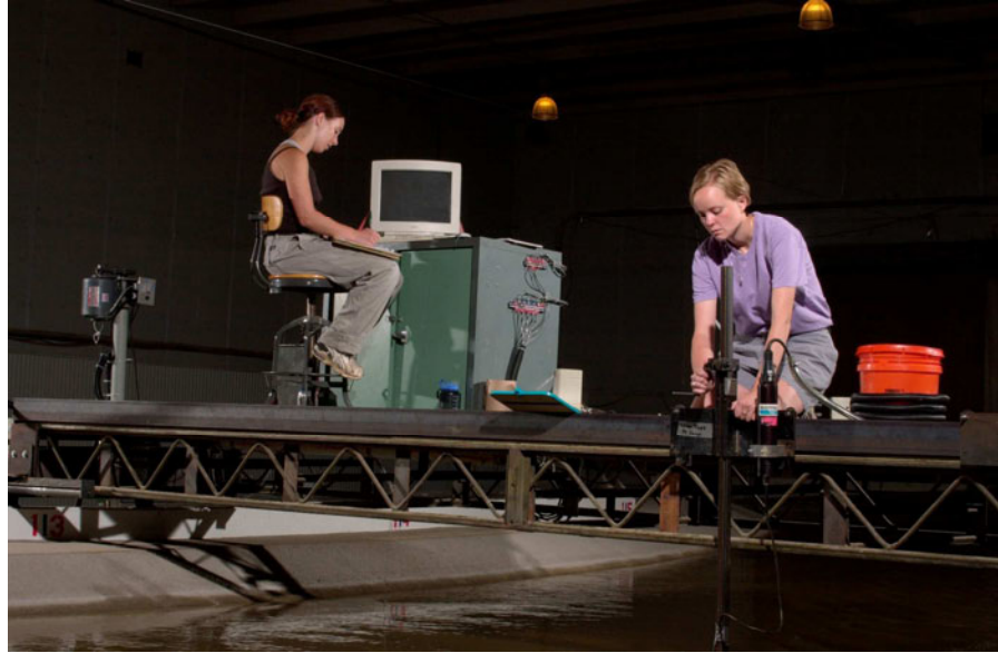
Figure A.17 Installation of ADV in Data Collection Cart
