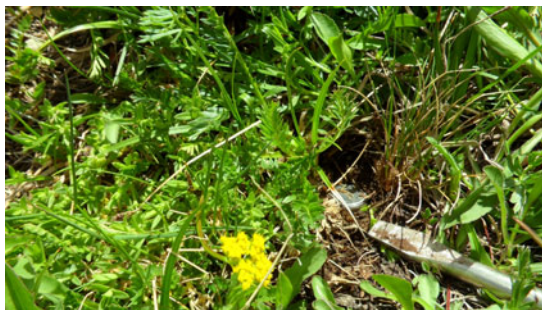
Figure 3. Temperature sensor (iButton) placement at mineral soil surface; iButton was slid under the Carex elynoides plant to the right, above the screwdriver tip.
