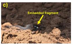
Figure 2— (a) Fragments from 7.62 by 54R steel core/steel jacketed bullet; (b) Fragments from 7.62 by 51 solid copper bullet; (c) Example of smoldering ignition from embedded bullet fragment.
