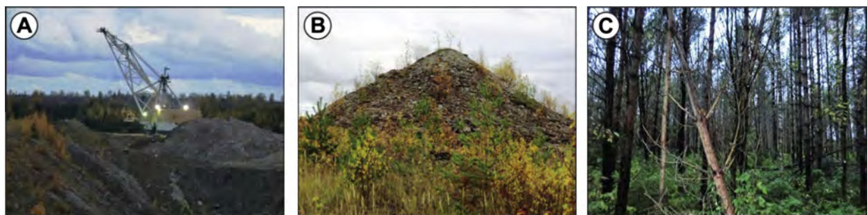
Fig. 3. Progression of reclamation on oil shale mined land in Estonia. Active mining site, where the overburden is being removed to expose the exploitable oil shale strata that generally is 5–35 m below the surface (A). Before leveling and shaping into a new landscape, piles of calcareous detritus dot the landscape (B). Since the 1960s, reclamation to woodlands, the previous landuse, has favored Pinus sylvestris L.; the stand shown is approximately 33 years-old (C). Specific information can be found in Laarmann et al. (in press). Photos by John A. Stanturf.
