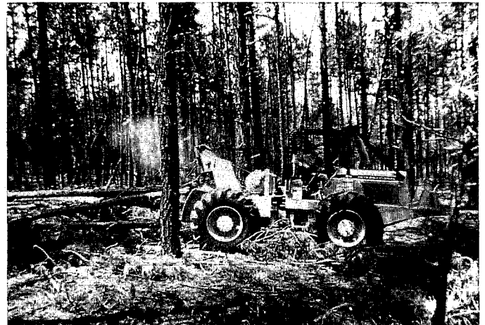
Figure 16.—Rubber tired skidders are too large to work well in seedbed preparation or slash disposal in partially cut stands.
