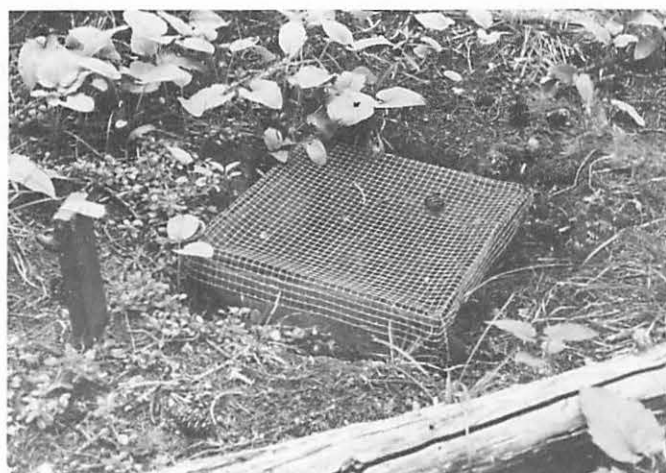
Figure 1.—One-foot-square wire seed trap in place. Fraser Experimental Forest, Colorado.
