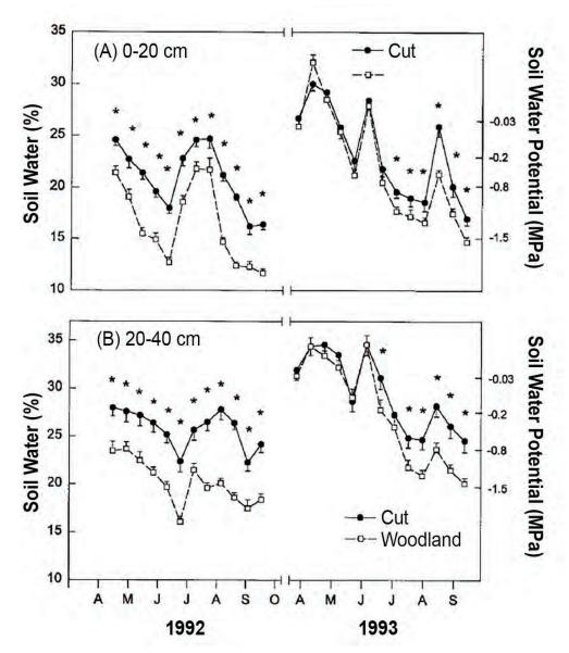
**Figure 2-47**—Gravimetric soil water content (percent soil water by weight) and soil water potential (less than -1.5 MPa = wilting point) in interspace soils from: (A) 0–20 cm and (B) 20–40 cm soil depth in cut and uncut Phase III woodlands. Soil water potentials were determined by predawn leaf water potential of sapling juniper trees left in the cut and uncut stands. Asterisks (\*) indicate significance differences on that sampling date (P < 0.05) (Bates et al. 2000).
