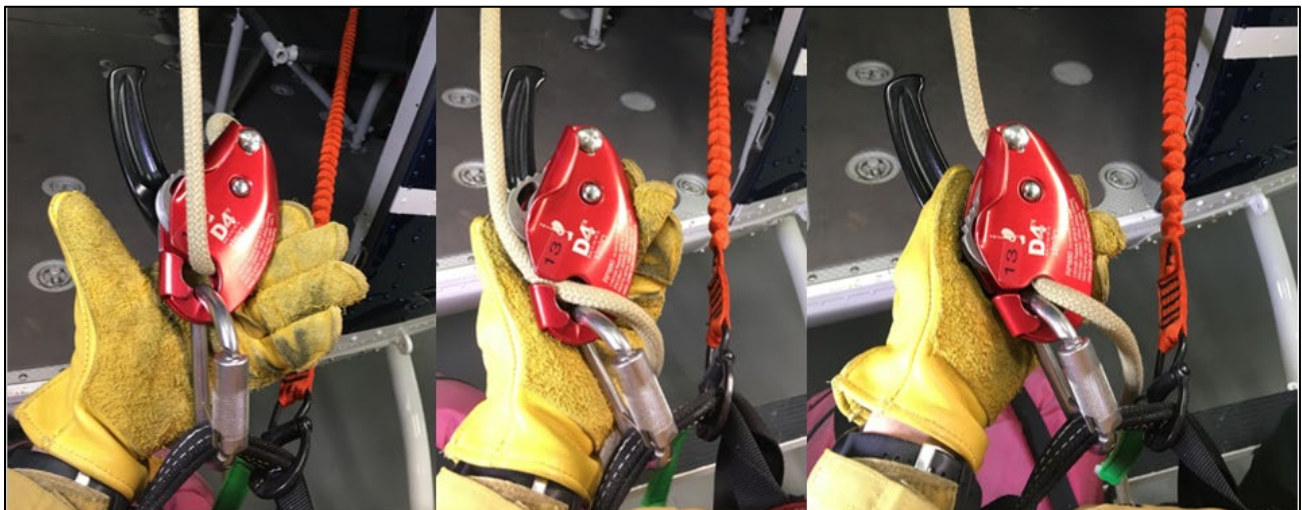
Rigged with the rope into the carabiner attachment point (CAP) three ways. From left to right: from anchor into the CAP, from anchor in the groove and out the CAP, rigged backwards and out the CAP.
