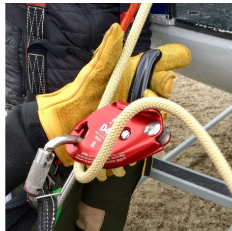
Descender rigged with rope between cover
