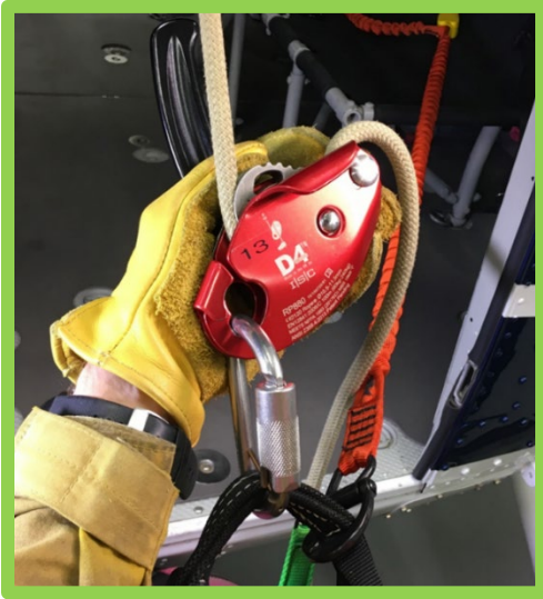
Descender rigged correctly
