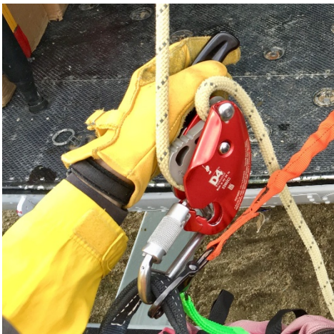
Descender rigged with carabiner captured in groove
