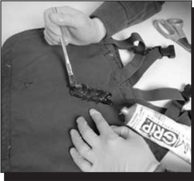
Figure 7—Spread Seam Grip over the entire hole.
