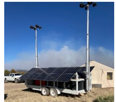
Option 2: Hybrid solar light + power trailer, 2022 Black fire, New Mexico. Photo by Margie Guzman.
